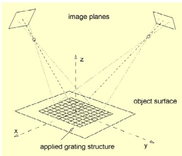
Fig. 1: Principle of 3D image correlation with 2 cameras
