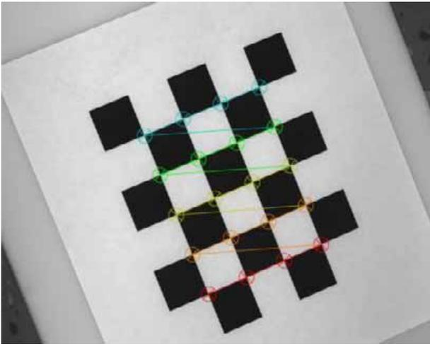
Fig. 3: Calibration plate with determined nodal points
