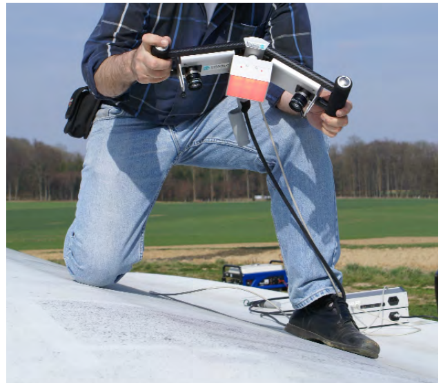
The Q-480 Handheld DIC for 'Point and Shoot' measurements.
